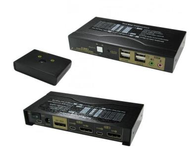
The 2/4 Port DisplayPort KVM allows you to switch between two or 4 computers using USB and DisplayPort connections. Supporting DisplayPort 4k@60Hz and 4:4:4 chroma subsampling, you can enjoy high quality 4k content. Comes complete with cables making it very easy to set up. Wired remote enables easy switching between two or four computers. Metal housing makes it very robust.
