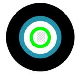
Universal Loose tube corrugated steel tape (CST) armoured optical fibre cables have been designed specifically for applications requiring a high degree of mechanical protection, including direct burial. These compact cables are extremely rugged, provide rodent resistance and are quick and easy to install.
